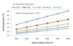
Fig. 3b: Variation in PV cell temperature of the PV/T air heater with solar irradiance and air mass flow rate
