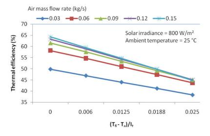
Fig. 5: Variation in PV/T air heater energy efficiency with air mass flow rate and ratio of air temperature rise to total solar irradiance.
