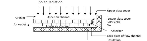
Fig. 2: Cross-section of double-pass PV/T solar air heater with fins (modified case)
