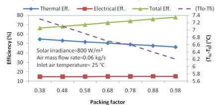
Fig. 7: Variation of efficiencies and rise in air temperature  $(T_{fo} - T_{fi})$  with packing factor.
