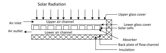
Fig. 1: Cross-section of double-pass PV/T solar air heater (base case)
