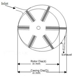
Fig.1 Air Turbine-Schematic Drawing
