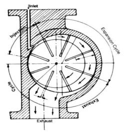
Fig.2 Air Turbine- Mode
