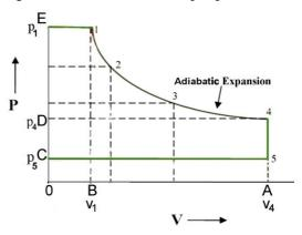
Fig. 3 Thermodynamic Processes (Isobaric, adiabatic and Isochoric Expansion)
