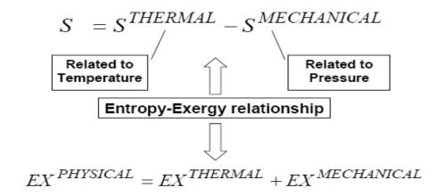
Fig. 2: Thermal and mechanical contributions to entropy property
