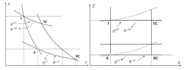
Fig. 3: Property of a symmetric cycle
