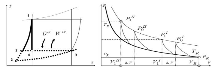
Fig. 5: mechanical exergy related to pressure
