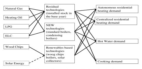
Fig. 1: Part of the RES of PP MarkAL Model (thermal residential sector)
