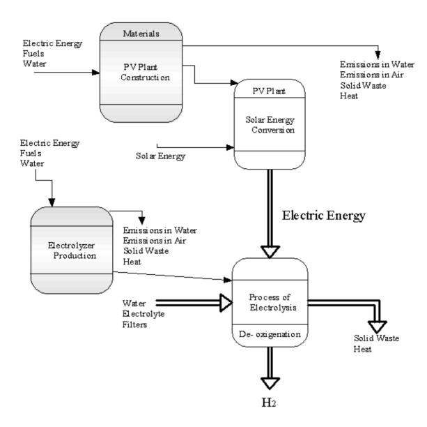
Fig. 2: Flow diagram and system boundaries of Photovoltaic productive cycle.
