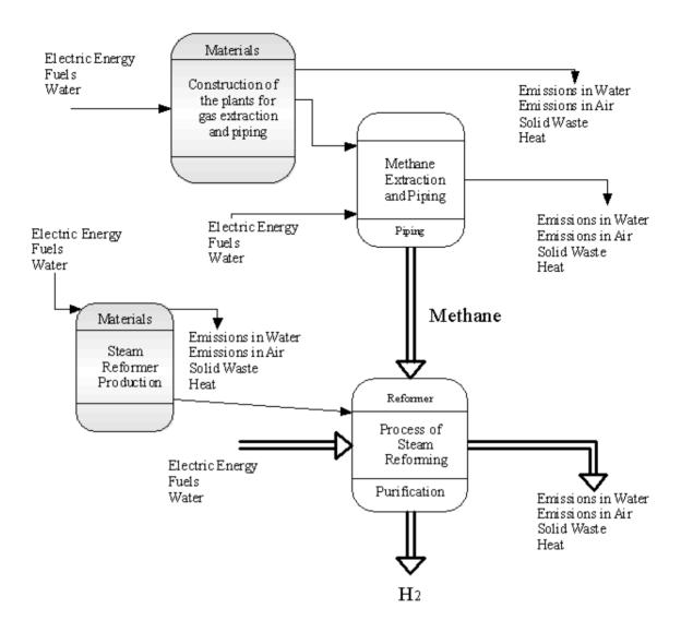
Fig. 1: Flow diagram and system boundaries for the methane steam reforming productive cycle.
